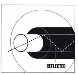
optical fiber, tie it in a knot, and light is still transmitted through it.
